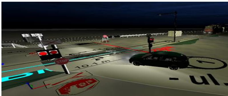
Fig. 6. Mutual position of vehicles 1.5 s before the collision – 3D view
