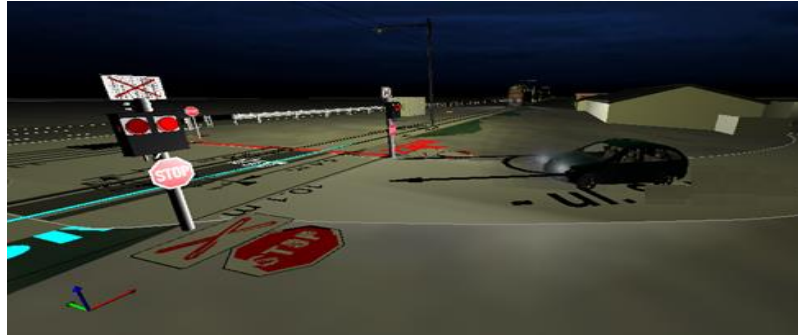
Fig. 5. Mutual position of vehicles 2.5 s before the collision – 3D view
